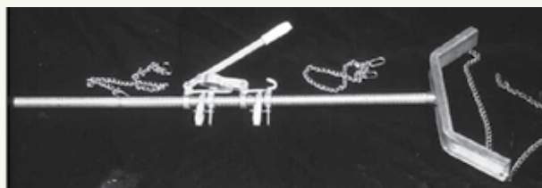
Figure 2. A mechanical calf extractor or puller which permits additional traction in pulling the calf in difficult births. It is designed to span the rear of the pelvis and insures pulling the calf at the correct angle and tension to avoid unnecessary injury to the cow and calf.
